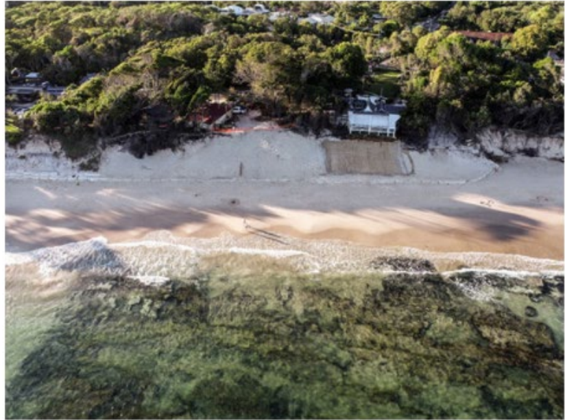
Aerial view of sandbag wall and beach nourishment in front of café and adjacent sandbag wall in front of Reflections Holiday Park – Clarkes Beach (January 2021)
